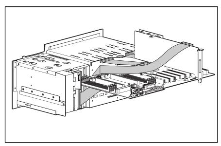
Figure 2-26. Array Controller removable media cable folding and routing diagram
